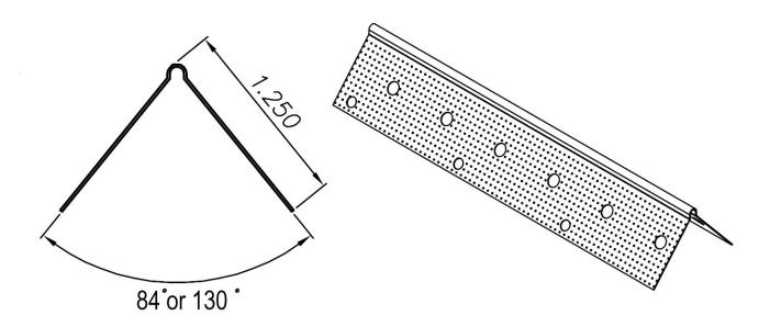
Our cornerbeads conform to Canadian steel standards They are available in standard 7, 8, 9, 10 and 12 foot lengths (90 and 135 Deg).
