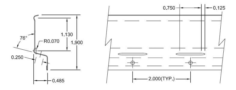
Our metallic resilient bars conform to Canadian steel standards. They are available in standard 12 foot lengths. They are an economical means of reducing noice transmission for wood or metal structual or load bearing partitions.
